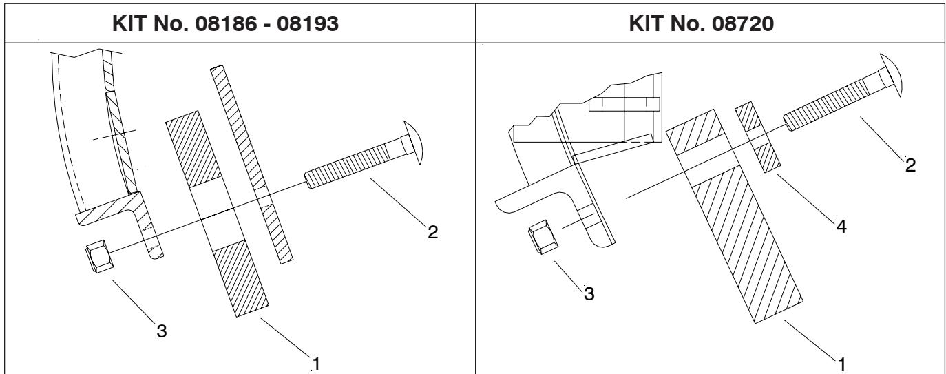
Remove existing steel cutting edge from snow plow. Position Rubber Cutting Edge on snow plow as shown and clamp in place by inverting snow plows original steel cutting edge. Fasten together using bolts and locknuts. For best results, runners must be removed. The rubber cutting edge is reversible for extended wear life. Best results will be obtained with wet, unpacked snow. Packed snow or ice cannot be removed with a rubber cutting edge.
