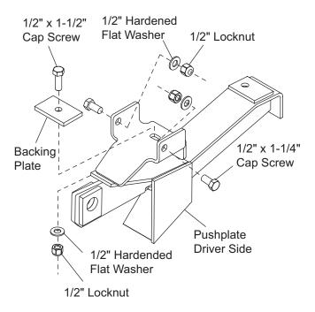
3. Insert a 1/2" x 1-1/2" cap screw down through a backing plate then through bottom of frame and the slot in the pushplate. The backing plate should span the inside bottom surface of the frame widthwise. Place a washer and locknut on the cap screw and hand tighten. Verify that the rear portion of the pushplate is in contact with the bottom portion of the frame.
