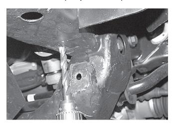
NOTE: Drill clearance can be obtained by turning the steering wheel so the front of the tire is away from side being drilled.
