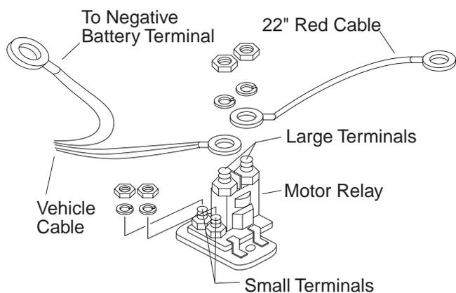
10. Attach the black wire from the vehicle cable to the negative (-) battery terminal.
