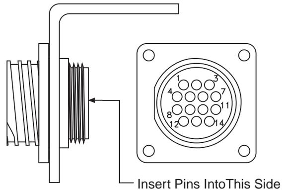
3. Mount the connector bracket to the vehicle with the supplied #6 sheet metal screws and washers. Secure the connector to the bracket with the 6-32 screws, lock washers and nuts.
