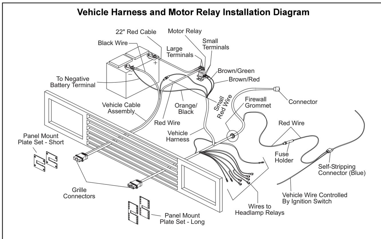
9. Attach the red wire from the vehicle cable to one of the large terminals on the motor relay. Secure with a lock washer and 5/16" jam nut.
