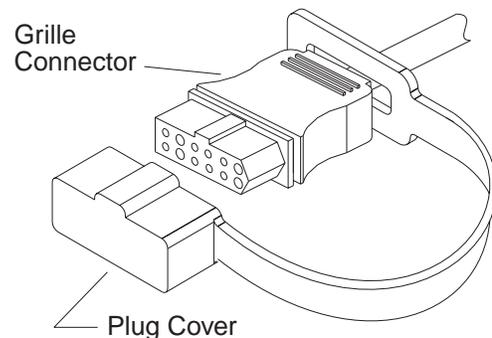
8. Route the vehicle cable through the grille at the selected location and through or around the radiator bulkhead to the motor relay. Be sure to avoid sharp edges and hot or moving parts.
