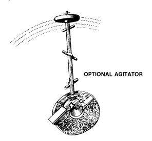
The CS-94 Series of seeder/spreaders have a two blade knife type agitator as standard equipment. An optional long wheel type agitator is available which will take care of air pockets in the hopper, mix up the material, and deliver it to the bottom knife type agitator. Order part number 420758 for the optional long wheel agitator.
