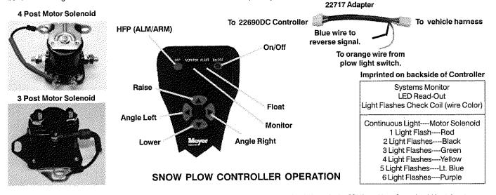
The snow plow should only be in operation when the vehicle ignition switch and the control switch are in the "ON" position. Care should be taken to ensure that the control switch is kept dry and free from moisture during normal operation.
