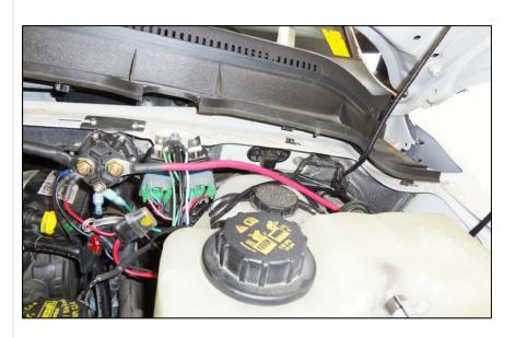
Install a solenoid and relays on the driver side (as shown on the picture). Ensure that solenoid is grounded; if necessary run 16-14 gauge wire from battery ground to the base of a solenoid.
