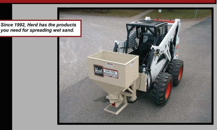
The Herd Salt/Sand Spreader is the Tool for Efficient Deicing. Ideal for Parking Lots and Walk-Ways, The model 750SSS couples the versatility of today's Skid Steers with the Durability that Herd is known for. Utilizing our unique agitator design, the Herd Salt/Sand Spreader is the most effective method of spreading any combination of sand *(wet or dry)*, salt, and calcium chloride.
